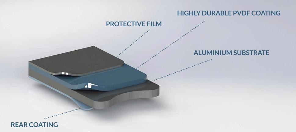
Futural is solid aluminium cladding panel that is A1 non-combustible to BS EN 13501-1 and suitable for any type of buildings at any height. Made from 5000 marine grade aluminium with PVDF coatings, it is highly durable and impact resistant, yet available in unlimited colour range with superior surface and weather resistance.
